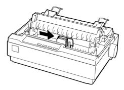
3. Turn the ribbon-tightening knob in the direction of the arrow to remove any slack from the ribbon so it is easier to install.
