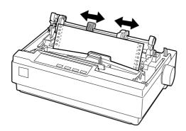
7. Make sure your paper has a clean, straight leading edge. Open the sprocket covers. Fit the first holes of the paper over the sprocket pins and then close the sprocket covers. Slide the right sprocket unit to remove any slack in the paper and lock it in place.
