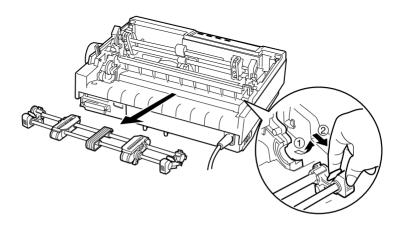
3. Move the tractor forward to the mounting slot at the top of the printer and tilt it into place as shown below. When you push the tractor onto the posts, you should feel the notches snap into place.
