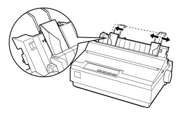
4. Slide a sheet of paper down firmly between the edge guides until it meets resistance. The printer loads the sheet automatically. The printer begins printing the self test.
