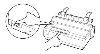
3. Slide the left edge guide until it locks in place at the guide mark. Next, adjust the right edge guide to match the width of your paper.
