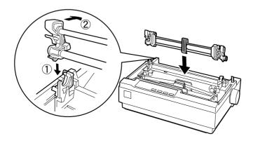
4. Release the sprocket units by pulling the sprocket locks forward.
