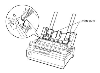
5. Slide the left paper guide so it is aligned with the triangle mark. Next, slide the right paper guide to roughly match the width of your paper. Slide the paper support midway between the paper guides.
