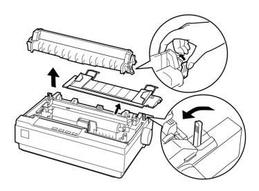
2. Squeeze the tractor's lock tabs gently and rotate the tractor up and pull it away from the printer.
