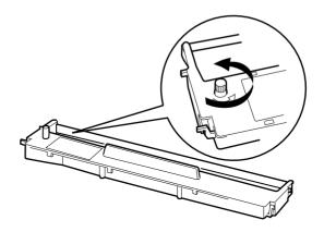
4. Insert the ribbon cartridge into the printer as shown; then press both sides of the cartridge firmly to fit the plastic hooks into the printer slots.
