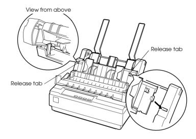
13. Slide the left edge guide to the center until it stops at the guide mark. Then slide the right edge guide to fit the size of paper you will use.
