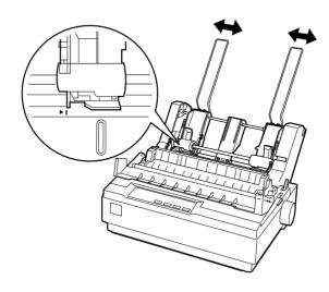
6. Pull the paper-set levers all the way forward until the paper guides retract and lock open to allow for paper loading.
