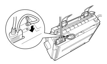
3. Plug the other end of the cable into the computer's parallel interface. (If there is a ground wire at the end of the cable, attach it to the ground connector at the back of the computer.)
