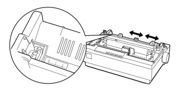
4. Make sure your paper has a clean, straight leading edge. Open the sprocket covers. Fit the first holes of the paper over the sprocket pins and then close the sprocket covers. Slide the right sprocket unit to remove any slack in the paper and lock it in place. Now the paper is in the paper-park position.
