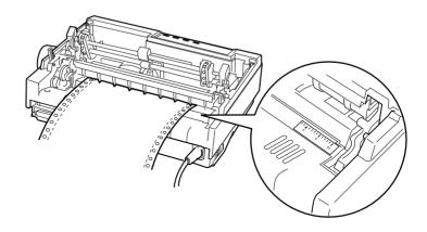
6. Slide the left sprocket unit so that its sprockets match the position of the holes in the paper and lock the unit in place. Then slide the right sprocket unit to match the width of your paper, but do not lock it. Move the paper support midway between the two sprocket units.
